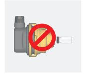
NOTE. Product codes with shut-off valve includes a paddle that extends 25 mm from the body valve. If needed, cut the exceeding part with a shear.
